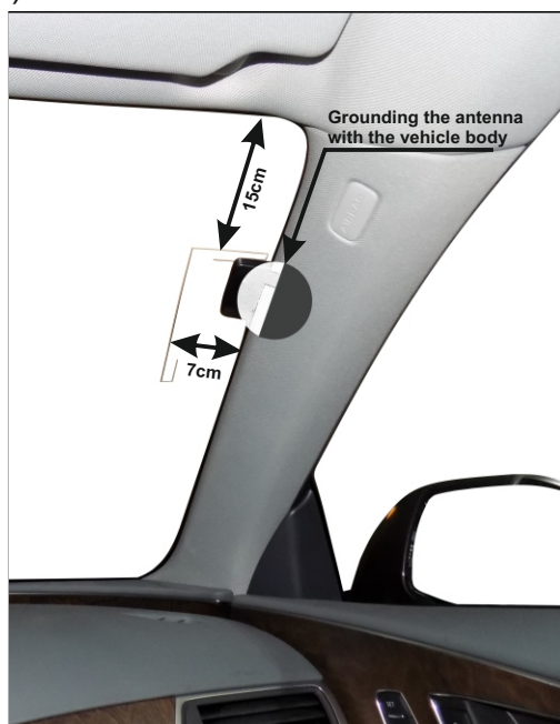
Example of mounting a DAB/DAB+ antenna
